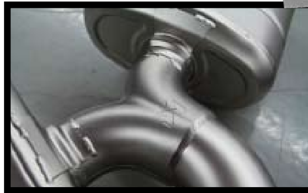
The quality and design that has gone into this system is beyond top-notch. Akrapovic even uses a cast-titanium split collector, something we have yet to see on any other exhaust system on the market.
