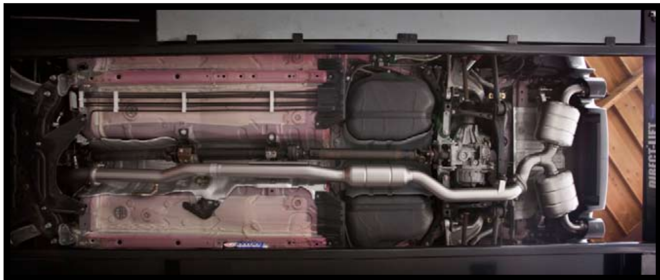
The Akrapovic exhaust follows the factory routing, ensuring proper fitment and placement.
